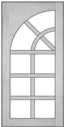
GP-LQC-2 Specify lite quantity below arch. Standard Framing: 2-3/8"
